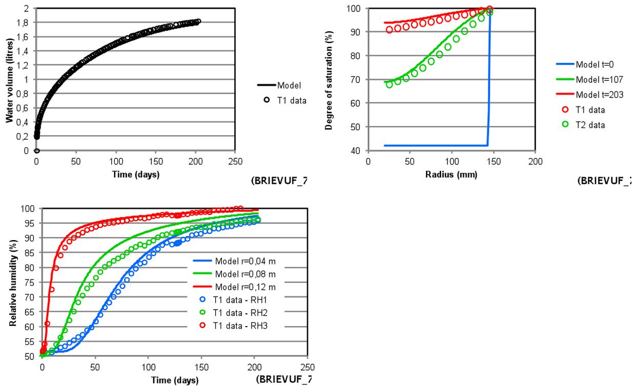
Figure 2 Experimental (symbols) and model results (lines) of cumulative water uptake (upper left), radial distribution of degree of saturation(upper right), and evolution of relative humidity (lower left).
