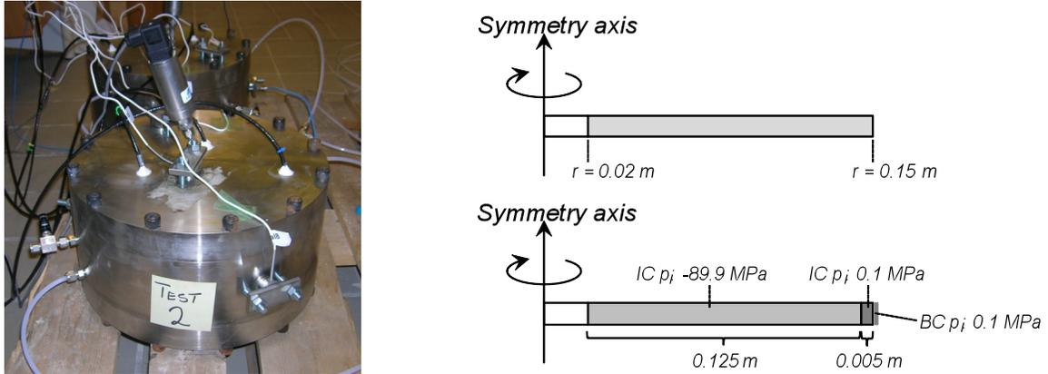
Figure 1. Test cylinder (left), model geometry (top right) and model initial and boundary conditions (bottom right).
