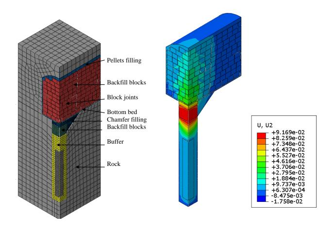
Example of modelling (Abaqus). Upwards swelling of bentonite buffer to the backfilled tunnel. Vertical displacements in meters.
