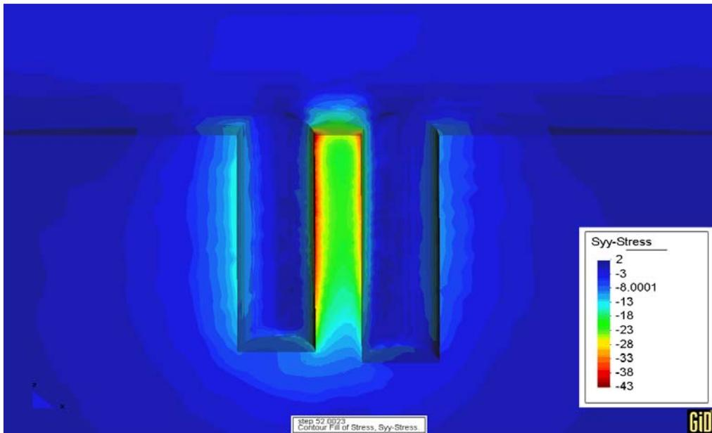
Code\_Bright simulation of the pillar stability test (APSE). The contours show the y-component (perpendicular to the tunnel) of the thermally induced stresses. In the pillar between the two deposition holes the maximum thermally-induced tangential stress is in the order of 40 MPa (SKB IPR-05-19).
