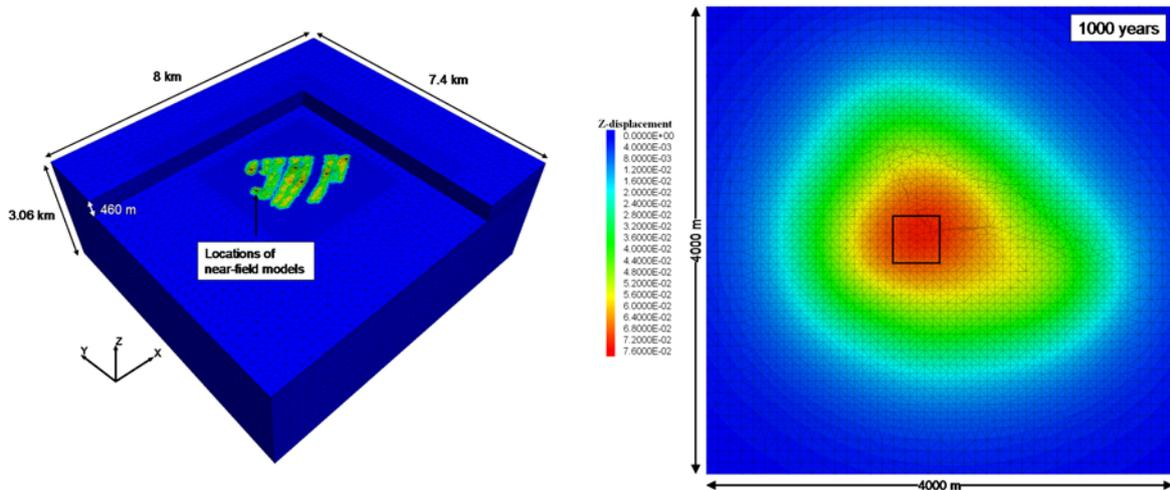
3DEC large scale thermo-mechanical analyses of Forsmark nuclear waste repository. Left: model outline with canisters positioned according to Forsmark layout at 460 m depth. Right: Heave of ground surface at time of maximum heave 1000 years after deposition. The maximum heave, averaged over the 400 m x 400 m square indicated in the figure, is 75 mm (SKB TR-10-23).
