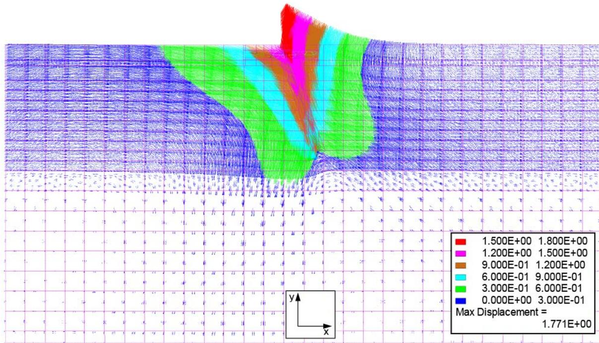
*Dynamic 3DEC earthquake modelling. The figure shows rock displacement vectors along a vertical cross section through a magnitude 6 earthquake 10 seconds after rupture initiation (SKB TR-08-11).*
