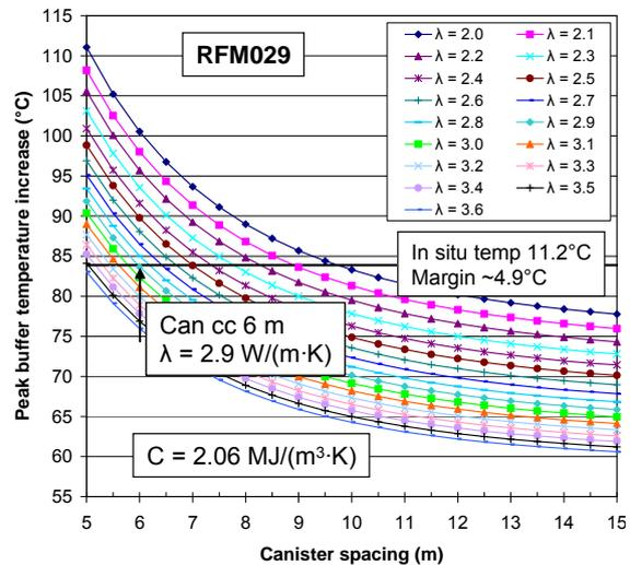
*Use of analytical solutions. Left: Contributions to local deposition hole rock wall temperature from nearby and distant canisters (SKB R-09-04). Right: Nomographic representation of relation between rock thermal conductivity, canister spacing and the peak increase of the temperature of the bentonite barrier surrounding the waste canisters (SKB TR-10-23).*
