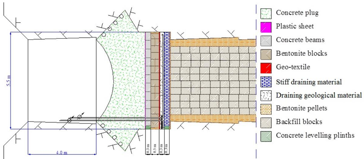
**Figure 1.** Schematic drawing of the plug design.
