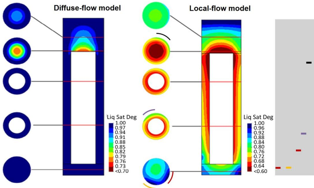
**Figure 1.** Contour plots showing the liquid saturation at the time when the buffer was excavated in the experiment. In the right-most panel a schematic drawing, showing the position of the local-flow zones on the deposition-hole wall is included. Where appropriate, the orientation of these zones is also shown around the horizontal cuts in the figure.
