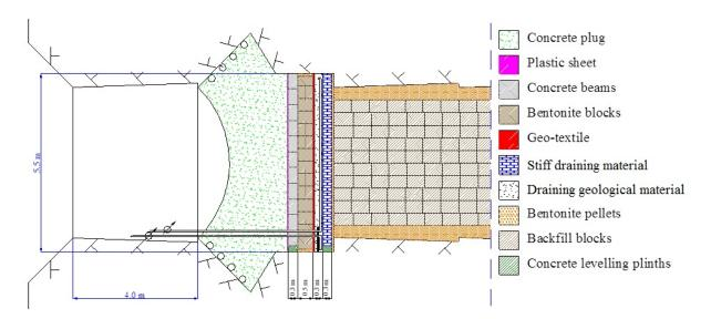
Figure 1. Schematic drawing of the plug design.
